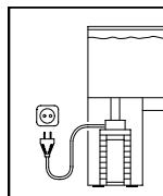
For your own safety, we recommend to form a drip loop with the connection cable to prevent any water running along the cable from intruding into the socket.
