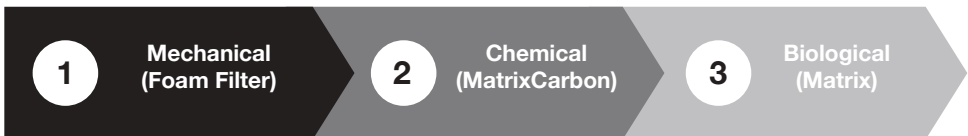
Figure 5: Layering Filtration Media (bottom to top)
