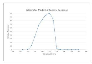
Fig. 1. Model 6.2 Spectral Response
